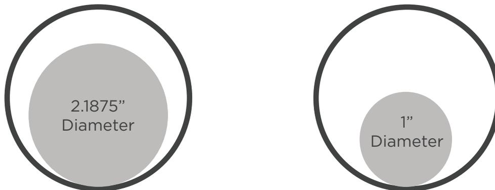
Since continuous rod contacts the tubing at the coupling, the diameter of the contact area is larger. 1" rod is shown in the figure above.
